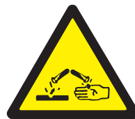
Caution, corrosive substance
